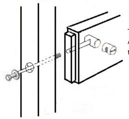
The barrel nut must be inline with the bolt. After insertion the bolt will thread through the nut to secure.
