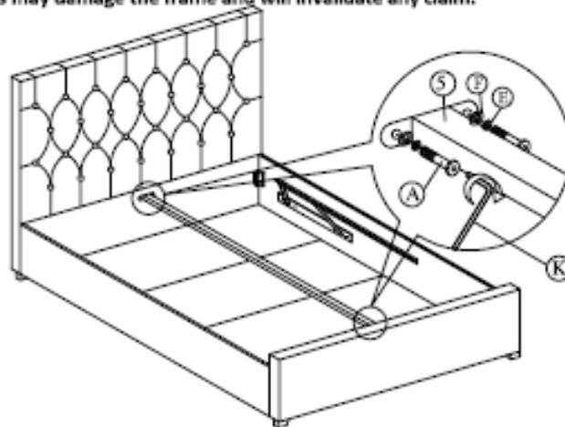
Step 8: Unscrew the Pre-attached hex-nut of gas spring (10) and attach it back again as shown. Please fully tighten the nut.
