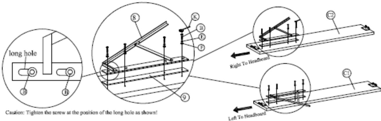
**Step 2: Attach the legs (4) to the headend (1) and footend (2). DO NOT use any power tools as this may damage the frame and will invalidate any claim.**
