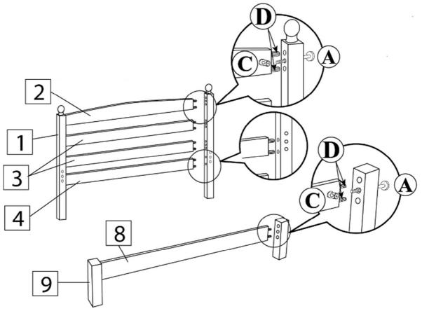
Step 2: Attach the side rails (5) using hardware parts A, C and D. DO NOT use any power tools as this may damage the frame and will invalidate any claim.
