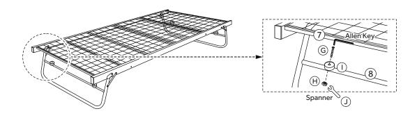
**STEP 7:** Hook the bar to the Trundle Leg (8) to lock it when in the open position. **DO NOT USE ANY POWER TOOLS AS THIS MAY DAMAGE THE FRAME AND WILL INVALIDATE ANY CLAIM.**
