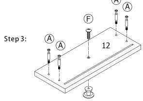
Insert hardware part (A) into the holes shown on the drawer front panel (12). Then attach hardware part (E) using hardware part (F).
