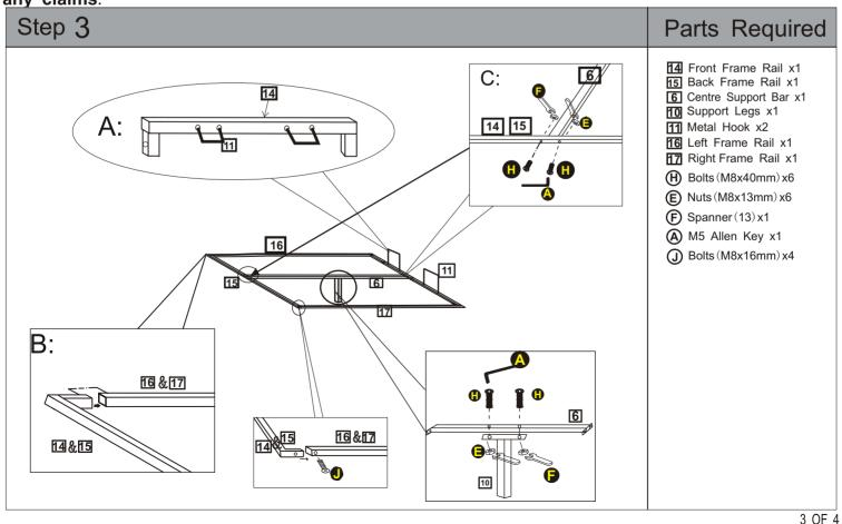
To attach the metal frame (14/15/16/17) and cross support bar (18) to the gas lift pre-fixed to the side rails, you will need to use hardware parts K, E and L with the M5 allen key (A) and the M14 spanner (F).
