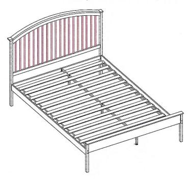
**Size**: 4FT, ASSEMBLE SIZE, L 2015 X W 1313 X H 1140 4FT 6IN, ASSEMBLE SIZE, L 2015 X W 1475 X H 1140 5FT, ASSEMBLE SIZE, L 2110 X W 1627 X H 1140
