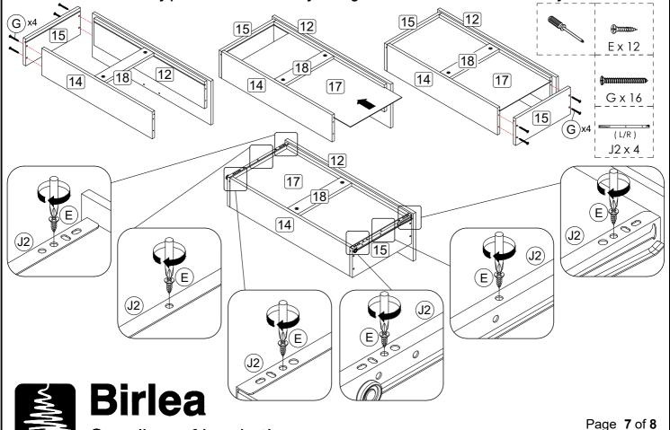
Step 12: Assemble the drawer in place along the drawer slides.
