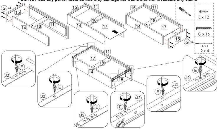
**Step 11:** Assemble the drawer components using hardware E, G and J2. In this step only show one of the drawers.
