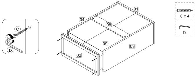
**Step 7:** Attach hardware I1 into panel (1), (2), (3) and (4) using hardware I2 with a screwdriver (not provided). **DO NOT** use any power tools as this may damage the frame and will invalidate any claim.
