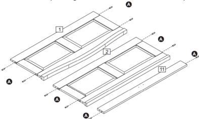
Step 3: Attach the left headend post (3) and right headend post (4) to the headend panel (1) and headend rail (11) using hardware parts H and M.
