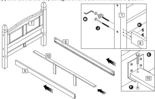
**Step 7**: Join the two sections together using hardware parts J, K and M. Secure the centre rail (10) using hardware parts E and F.
