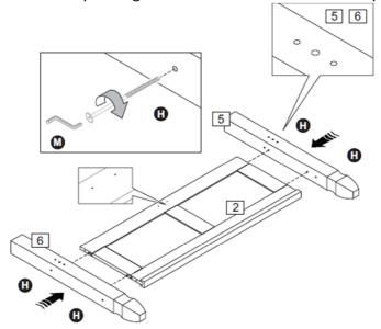
Step 5: Secure hardware part L using hardware part C and a screwdriver (not provided). DO NOT use any power tools as this may damage the frame and will invalidate any claim.
