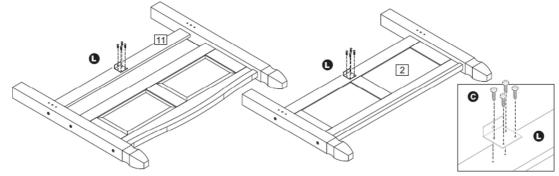
Step 6: Attach the side rails (9) using hardware parts J, K and M. Secure the centre rail (10) using hardware parts E and F.
