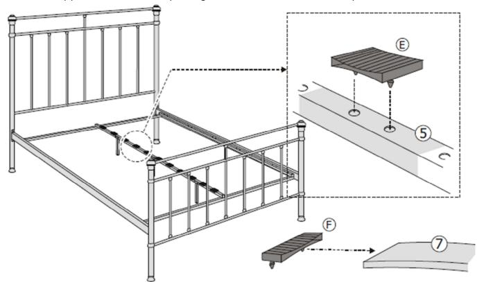
Step 6: Insert the slats (7) to hardware part E and press firmly into the side supports (3). Insert hardware part I.
