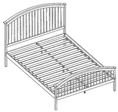
**Size**: 4FT, ASSEMBLE SIZE, L 2015 X W 1313 X H 1140 4FT 6IN, ASSEMBLE SIZE, L 2015 X W 1475 X H 1140
