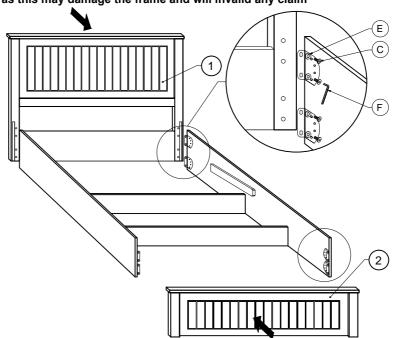
Step 3: Attach hardware part (O) to the footboard (2) and siderails (5) and (6) using hardware part (D) and (F). Attach the gas spring (16) to the gas lift mechanism (15) using the included nut. Then attach the gas lift mechanism (15) to the siderails (5) and (6) using hardware parts (E), (D) and (F).
