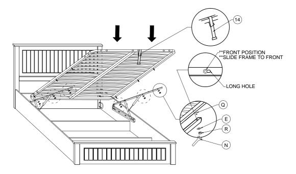
**Step 7**: Insert the Front, Centre & Back bottom panels (3) and (4) in the shown directions. **Warning: DO NOT use any power tools as this may damage the frame and will invalid any claim**
