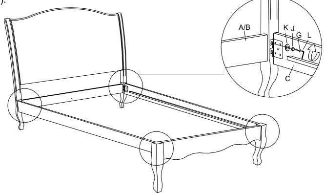
2 Insert JCBC M6 X 15mm (I) to L/Bracket (O) to Center Support (D) connection Headboard (A)/Footboard Panel (B) by Allen Key M4 (M).
