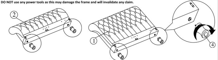
Step 3: Attach the pump mounting bracket (8) and bracket base (9) to the headend (1) and footend (2) using hardware parts B, D, E and J. DO NOT use any power tools as this may damage the frame and will invalidate any claim.
