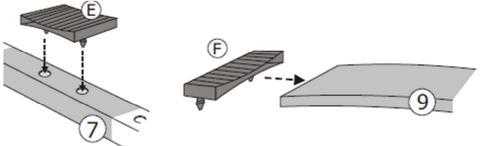
Step 8: Place the slats (9) into hardware part E then press hardware part F firmly into the side supports (5). DO NOT use any power tools as this may damage the frame and will invalidate any claim.
