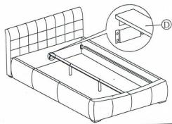
Step 4: Insert the sprung slats to both end of slat middle holder(1) before attaching slat end holders(2) to the other end of sprung slats. Having done this, press down the middle holder(1) and end holders(2) to the siderail support and center rail. Repeat the above for balance rows.
