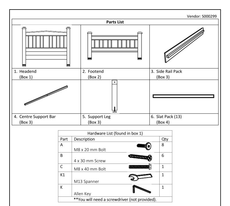
Step 1: Attach the side rails (3) to the headend (1) and footend (2) using hardware parts A and K. DO NOT use any power tools as this may damage the frame and will invalidate any claim.
