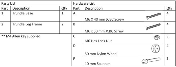
Step 1: Attach the base legs (2) to the base frame (1) using hardware parts A and C.
