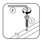
Step 6: Attach the Metal Side (10) to panel (3) and (4) using hardware I and F.Attach the Metal Side (10) to Metal Middle (11) using hardware J and F.DO NOT use any power tools as this may damage the frame and will invalidate any claim.
