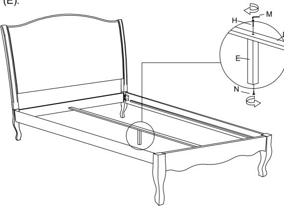
4 Use Spacer (Q) to adjust Slat (F) space. Insert CSK M4 X 32mm (P) to Bed slat (F) connection Side Rail Shelf (C).
