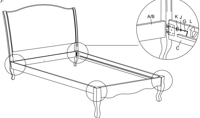
2 Insert JCBC M6 X 15mm (I) to L/Bracket (O) to Center Support (D) connection Headboard (A)/Footboard Panel (B) by Allen Key M4 (M).
