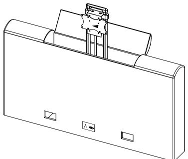
TV mounting bracket is factory fitted. If your TV has a 75 x 75mm VESA fixing remove it & fit TV directly to column bracket.
