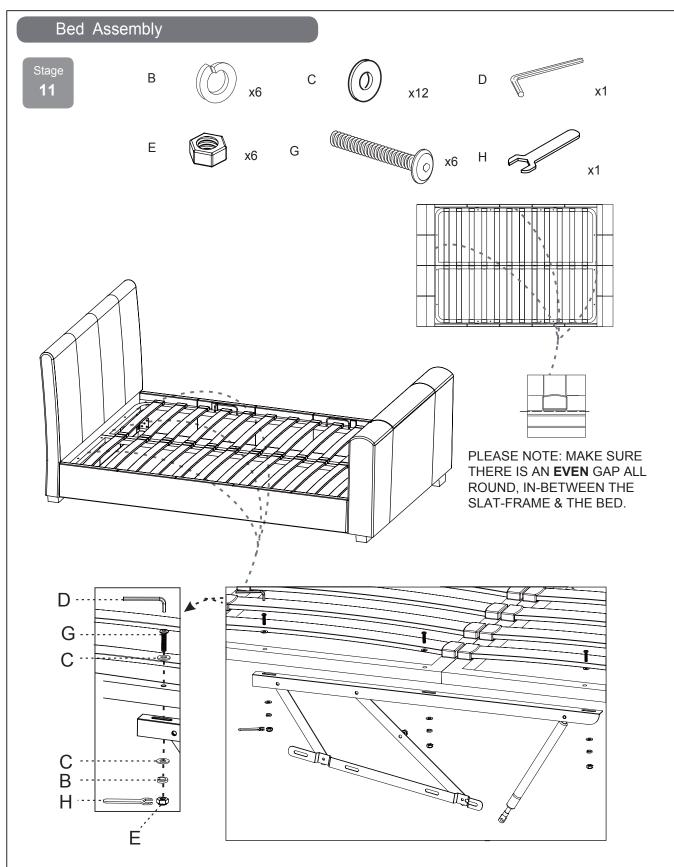
Use fixings (E), (C), (B) & (G)- tighten the bolt by using allen key (D) with spanner (H). NOTE: Do not fully tighten all the bolts before confirming the metal frame is in correct position. Frame must be in the centre of bed in length & width. Check frame is not likely to touch either headboard or footboard when lifting or closing. Tie lifting strap to opening side.
