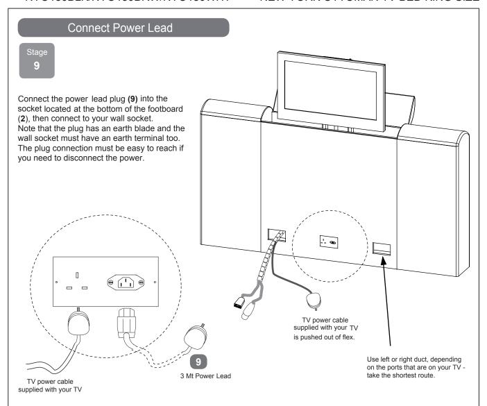
Plug the TV power cable into the socket at bottom of footboard then connect your own media cables as required.
