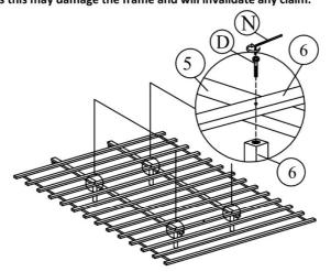
step 31 :Place the slat section into the assembled frame and secure to the headend (1) using hardware part H and a screwdriver (not provided). Secure the solid slats (4) using hardware part C and a screwdriver (not provided).
