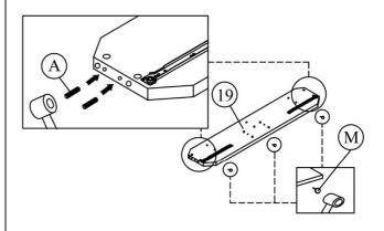
Step 9 : Insert hardware parts A and M to the drawer center frame (20) using a small mallet ( not provided).
