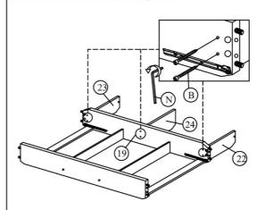
Step 20: Insert the drawer frame support (25) to the set up frame. Secure the drawer frame support (25) using hardware part B and N. DO NOT use any power tools as this may damage the frame and will invalidate any claim.
