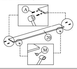
Step 10: Insert hardware parts A to the drawer frame support (21) using a small mallet ( not provided).
