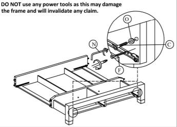
Step 25: Insert hardware part I to the side rails (3) using a screwdriver (not provided).
