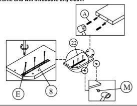
Step 14 :Attach the drawer runner from pack 2 (8) to the drawer frame divider 2 (23) using hardware part E and screwdriver(not provided). Insert hardware parts A and M to the drawer frame divider 2 (23) using a small mallet ( not provided).
