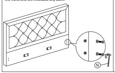
Step 29: Attach the headend (1) and footend (2) using the pre-assembled screws and hardware part N.
