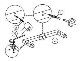
Step 23 : Attach the footend (2) to the frame (24) using the screws and hardware part I , J , K and N  $\,$
