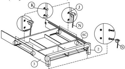
Step 28: Loosen the pre-inserted screws on the headboard (1) using hardware part N.
