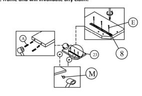
Step 15 :Attach the drawer runner from pack 2 (8) to the drawer center divider (24) using hardware part E and screwdriver(not provided). Insert hardware parts A and M to the drawer center divider (24) using a small mallet (not provided). the flip drawer runner from pack 2 (8) to the other side and repeat the same step.
