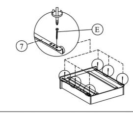
Step 5: Attach the drawer runner from pack 2 (8) to the drawer frame (18) using hardware part E and screwdriver( not provided).
