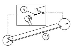
Step 17: Insert hardware parts A to the drawer frame support (26) using a small mallet ( not provided).
