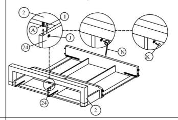
Step 24: Secure the frame using hardware parts C, F, N and O with a screwdriver (not provided).
