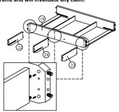
Step 19 : Secure the frame using hardware parts B and N .  $\mbox{DO NOT use any power tools as this may damage}$
