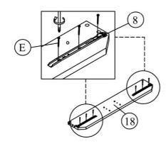
Step 6: Insert hardware parts A and M to the drawer frame (18) using a small mallet ( not provided).
