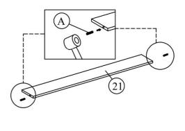
Step 11: Join together the drawer frame (18 & 19), drawer center frame (20) and drawer frame support (21).
