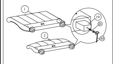
Step 15 : Attach the headend (1) and footend (2) using the pre-assembled screws and hardware part P.
