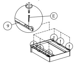
Step 5: Attach the drawer runner from pack 2 (10) to the drawer frame (16) using hardware part E and screwdriver( not provided). DO NOT use any power tools as this may damage the frame and will invalidate any claim.
