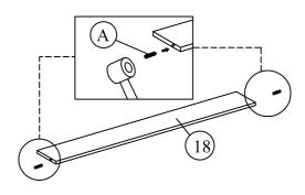
Step 9 : Join together the drawer frame support (18) and drawer center frame (17) to the drawer frame (16) .
