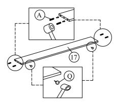
Step 8 : Insert hardware parts A to the drawer frame support (18) using a small mallet ( not provided).
