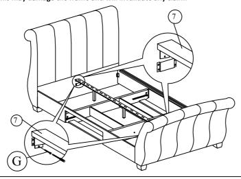
Step 18: Tighten all the 4 corner , follow by assembly of the slat holders with LVL slats as shown. Insert the drawer as shown.
