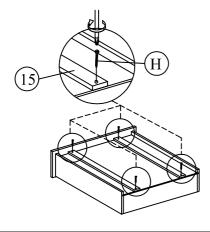
Step 4: Attach the drawer runner from pack 1 (9) using hardware part E and screwdriver( not provided).
