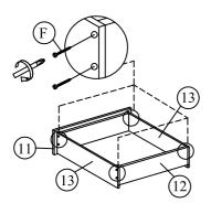
Step 2 : Slide the drawer bottom panel (14) into position on all Two drawer . Secure with hardware part L and small mallet ( not provided). DO NOT use any power tools as this may damage the frame and will invalidate any claim.
