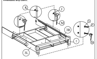
Step 14 : Attach the leg with headend (1) and footend (2). Using hardware part H.
