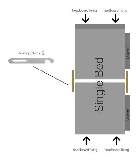
**Step1.** Connect each half of the bases together using joining bars.
