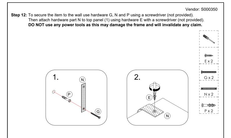
PLEASE NOTE that wall fixings are not supplied as different wall materials require different fixing devices. You must use fixings devices suitable for the type of wall you intend to mount product to. Ensure the head of any screw used has a diameter greater than the mounting hole and the fixing is safe and secure before use.
