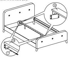
Step 5: Tighten all the 4 corners, followed by assembly of the slat holders with slats as shown.
