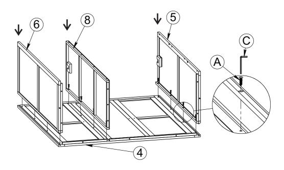
Note: All screws must install according to the working hole.
