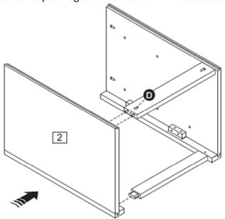
Step 6: Attach the top panel (1) and secure using hardware part D, then secure the bottom front frame (6) into position using hardware part B. You will need to use a screwdriver (not provided). DO NOT use any power tools as this may damage the frame and will invalidate any claim
