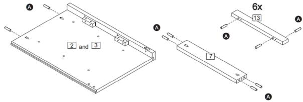
Step 4: Attach the bottom front frame (6) and rear base plinth (7) to the left panel (3) using hardware part D and a screwdriver (not provided).
