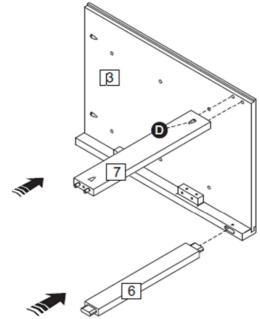
Step 5: Attach the right panel (2) using hardware part D and a screwdriver (not provided). DO NOT use any power tools as this may damage the frame and will invalidate any claim
