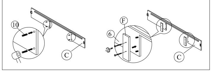
Step 3: Attach side rail (C) to headboard (A) and footboard (B) by pushing the bracket down to fit it.
