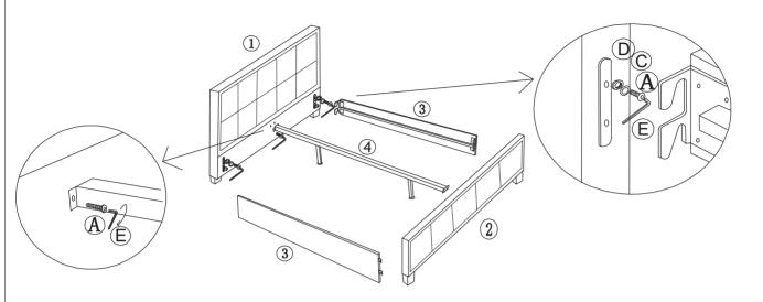
Step 4: Assemble the slats (6) as shown in the diagrams below then push all of the plastic cap's firmly into the side rails (3) and centre rail (4)
