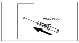
STEP 3: Put the screw in the wall plug hole
