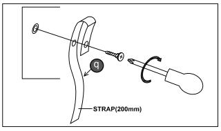
**NOTE:** Wall fixing are not supplied with this product as different devices (such as Rawl plugs on brick work). You must use fixing devices suitable for the type of wall you intend to mount this product to. Please ensure that the head of any screw used has a diameter greater that the diameter of the mounting hole on the product and than the fixing is safe and secure before use.
