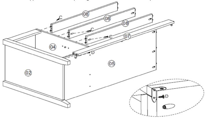
Step 7: Attach the right panel (3) using hardware part C and D, then attach hardware part H using hardware part D. You will need to use a screwdriver (not provided).
