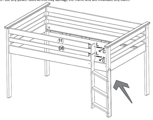
Step 7: Secure the ladder in position using hardware parts C and L. Attach the support (10) using hardware part G and a screwdriver (not provided).
