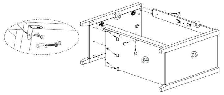
Step 7: Attach the top panel (1) using hardware part B and a screwdriver (not provided). DO NOT use any power tools as this may damage the frame and will invalidate any claim.
