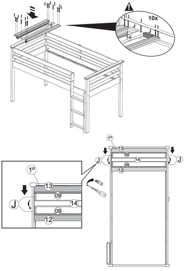
Step 10: Attach the remaining slats (14) and runner slat (13) using hardware parts I and J with a screwdriver (not provided).
