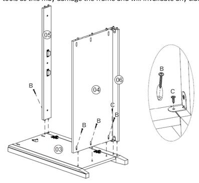
Step 6: Attach the left panel (2) using hardware parts B and C with a screwdriver (not provided). DO NOT use any power tools as this may damage the frame and will invalidate any claim.
