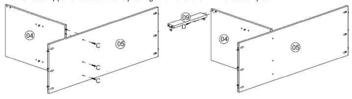
Step 5: Attach the left panel (2) using hardware parts C and D with a screwdriver (not provided). DO NOT use any power tools as this may damage the frame and will invalidate any claim.
