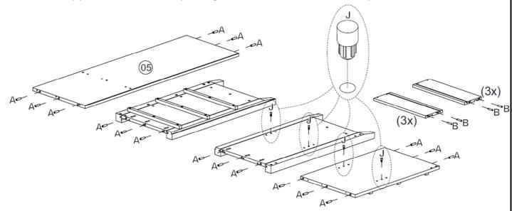
**Step 3**: Assemble the drawer components using hardware parts C, D, E and G with a screwdriver (not provided).
