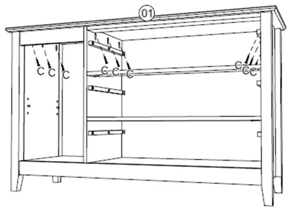
Step 9: Connect the back panels (16) with the spine (17) and secure in position using hardware part F and a small mallet (not provided).
