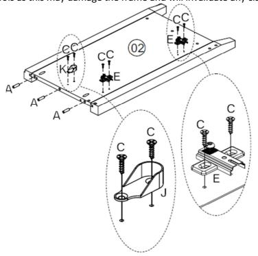
Step 3: Insert hardware part A to the right panel (3) using a small mallet (not provided). Attach hardware parts E and K using hardware part C and a screwdriver (not provided).
