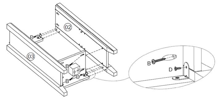
Step 7: Attach the top panel (1) using hardware part B and a screwdriver (not provided). DO NOT use any power tools as this may damage the frame and will invalidate any claim.
