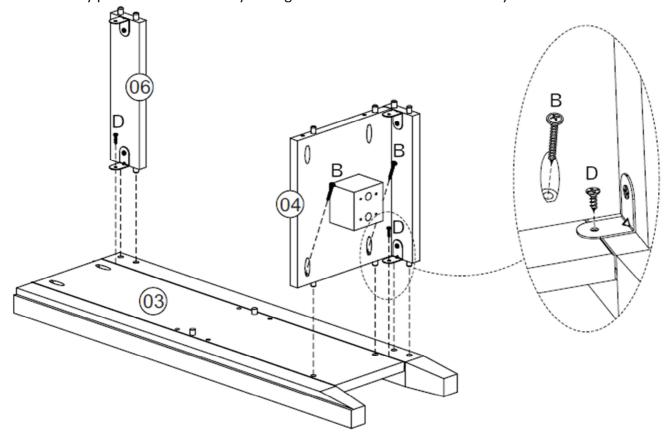
Step 6: Attach the left panel (2) using hardware parts B and D with a screwdriver (not provided). DO NOT use any power tools as this may damage the frame and will invalidate any claim.
