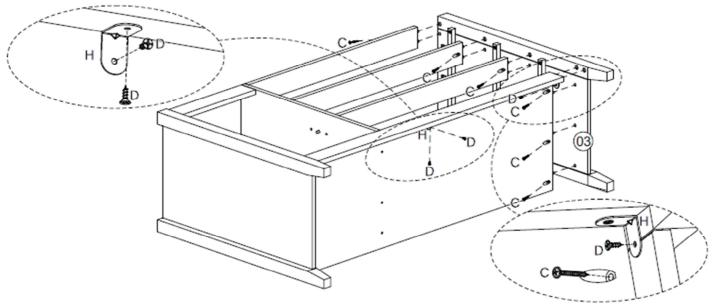
Step 8: Attach the top panel (1) using hardware part C and a screwdriver (not provided). DO NOT use any power tools as this may damage the frame and will invalidate any claim.
