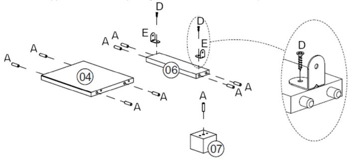
Step 4: Attach the support block (7) to the base panel (4) using hardware part I and a screwdriver (not provided).
