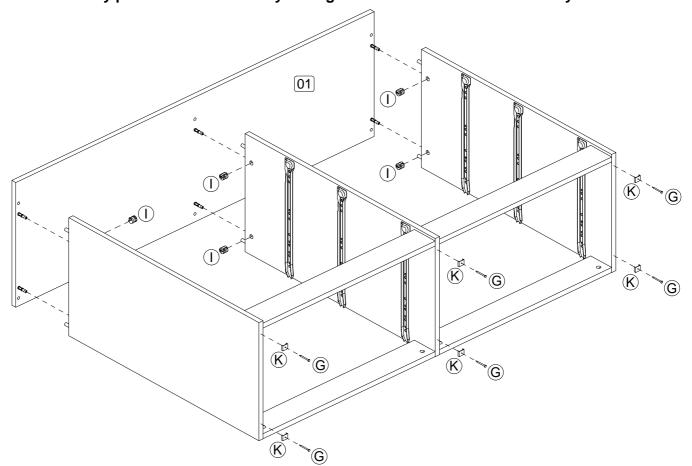
**Step 8:** Connect the back panels (15) using the spine (18) and secure using harware part G and a small mallet (not provided).
