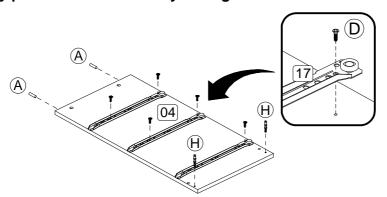
**Step 5:** Insert hardware parts A, H and N using hardware part J, a small mallet and a screwdriver (not provided).
