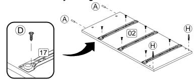
**Step 3:** Attach three drawer runners (17) to each side of the centre panel (3) using hardware parts M and a screwdriver (not provided). Insert hardware part A using a small mallet (not provided).
