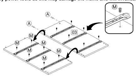
**Step 4:** Attach three drawer runners (17) to the right panel (4) using hardware parts D and a screwdriver (not provided). Insert hardware parts A and H using a small mallet and screwdriver (not provided).
