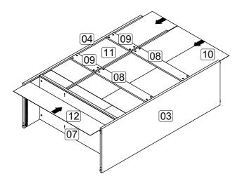
Step 4: Attach side panel (3), (4) and center panel (5) to top panel (1) then center panel (6) to middle panel (7) using hardware A1 and A2 with a screwdriver (not provided).
