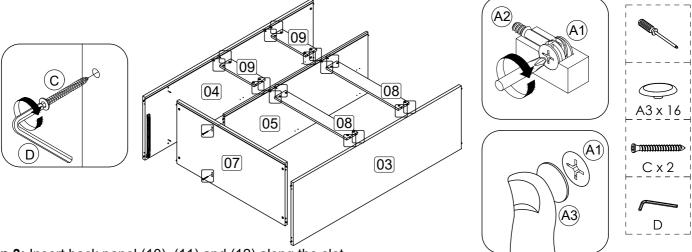
Step 3: Insert back panel (10), (11) and (12) along the slot.
